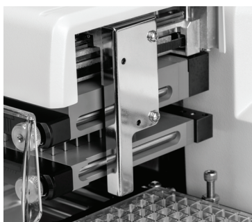
The Agilent BioTek Verify module is built in above the manifold and determines the fluid volumes in each well following dispense and aspirate cycles.
